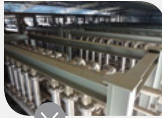
The **ROSS™** System is a simplified, yet robust solution for the treatment of oilfield produced water. Using CeraMem® ceramic membrane technology, this system provides removal of oil and silica as well as softening of the water simultaneously in a fully modular system.
