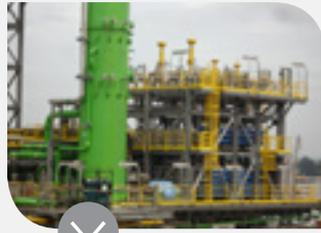
The **SULPHATE REMOVAL PLANT (SRP)** is used to extract sulphates from seawater prior to injection. The SRP uses nano-filtration membranes to remove the sulphates while leaving the other salts unaffected, thus maintaining the stability and permeability of the formation clays.
