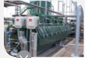
**AUTOFLOT™** is a Mechanical Induced Gas Flotation (IGF) separator. Induced Gas Flotation separates oil from produced water or other oily water streams with a low retention time. An hydraulic version of our IGF is also available depending on the application.
