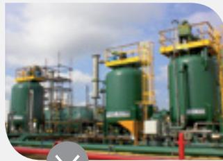
**POWER CLEAN™** nutshell filters are effective for the removal and treatment of hydrocarbons and suspended solids from produced water and petrochemical applications. Power Clean™ filters remove 98% of all filterable contaminants to recover more oil in a rugged, compact design.
