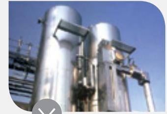
**MPPE** (Macro Porous Polymer Extraction) systems remove dissolved and dispersed hydrocarbons such as aliphatic, aromatic, polyaromatic and halogenated compounds. The technology is robust and compact, particularly adapted to offshore constraints and gas field produced water.
